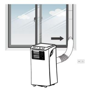
Step 7: Manually open the louvre on the front of the portable air conditioner. The internal louvres can also be moved manually from left to right to direct the airflow.
